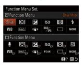
Up to 12 frequently used functions can be registered in both Still and Movie to the Fn (Function) button separately.
